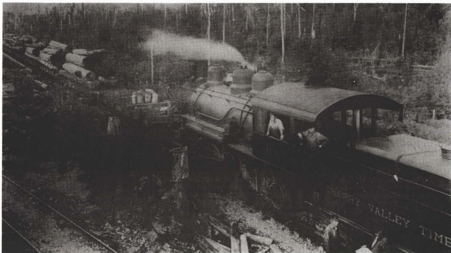
A MAIN-LINE rod engine, bringing logs down to the Milwaukee Railroad. The photo was made on Stillwater Hill near Lake Joy. Engineers backed their engines down a hill. With the front end elevated, hotter steam could be kept in the steam dome.
